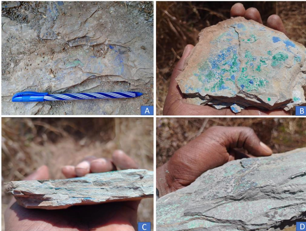
Figure 6: Copper mineralization (PR14701): A and B) Azurite (bleu) and malachite (green) occurred in bedding plan of the dolomitic shale; C and D) Azurite and malachite precipitated in fractures and bedding plan.
